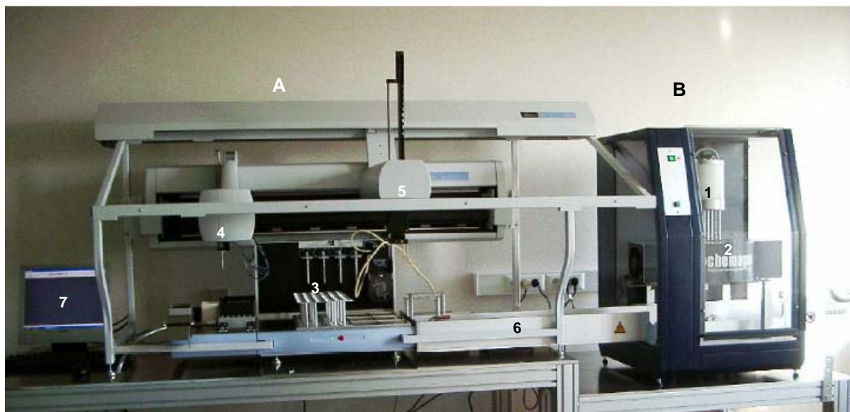
Figure 4: Integration of the chemagic MSM I extraction robot (B) with the Perkin Elmer MPEX liquid handler (A). Note that the 12 rod head (1) is situated just above the electromagnetic ring (2). After the tubes in the racks (3) have been filled by the 8-tip pipetting system (4), the racks are picked up by the gripper (5) and placed on the chemagen array (6). This array can move along the x-axis in order to place the correct tubes under the magnetic rod head. The rods can move along the y-axis and thus descend into the fluids in the tubes to attract the beads together with the DNA or to rotate and thus homogenize the solution. The entire process is controlled by one computer (7) with both software packages installed.
